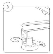
Bring the arm to the base and slide in from behind into the cup. Once in place, using the 1 x 4mm allen key lock arm into cup. You then clip the plastic cover over the base for a stylish finish.
