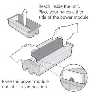
To lower the power module depress both the side buttons.
