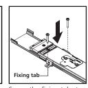
Screw the fixing tabs to the floor as shown.
