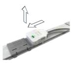
3. To remove, press button to disengage. Push forward and lift up to remove.
