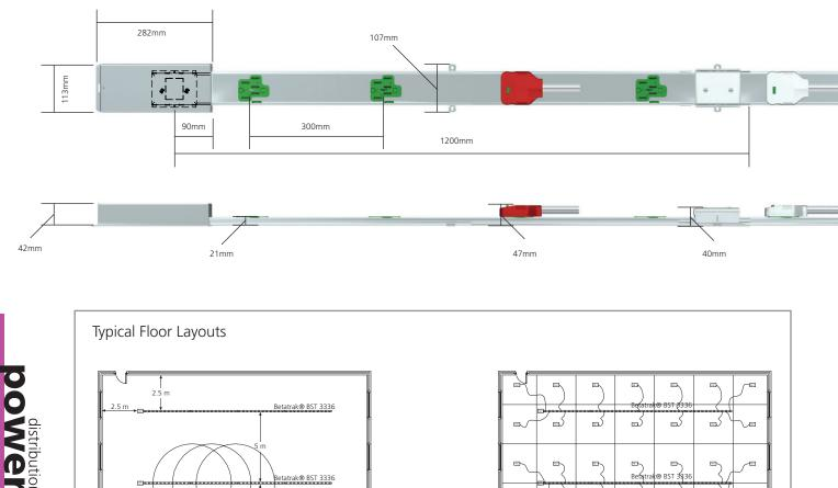
**m** <u>-</u> BST 33 atrak® BST 3336 5 ک\_ 5 ر ا \_ (0) Area cov by tap off lead Ξh (a.) Benatrak® BST 333 **11** etatrak® BST 3336 (m) 21 Busbar Floor Boxes 3m tap offs provide full coverage when busbar is laid out on 5m Typical layout: 1 floor box for every 10m<sup>2</sup>. centres
