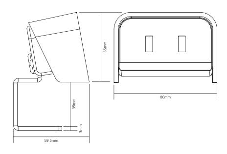
Note: Chip comes complete with bespoke C clamp fixing for desk thickness 15mm to 35mm.
