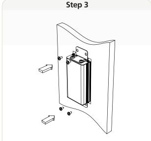
Secure the module to the inside of the furniture using a suitable fixing screws (not supplied). Take care not to over tighten the screws.
