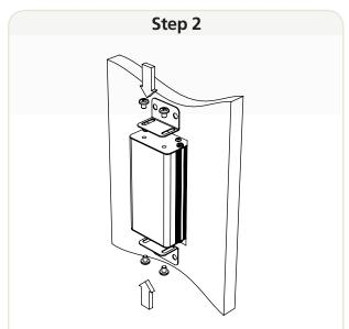
Fix the L shape bracket to the module using the fixing bracket screws (fig. 03). The brackets must be tight against the furniture surface before tightening.
