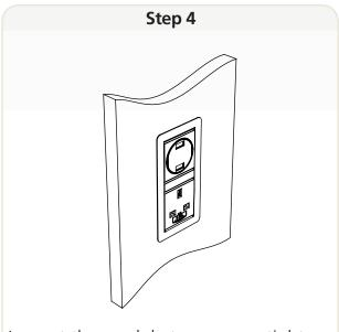
Inspect the module to ensure a tight and consistent fit has been achieved.
