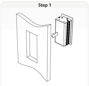
Remove the L shape fixing brackets (fig. 02) before placing the back of the module through the pre-cut hole in the furniture.
