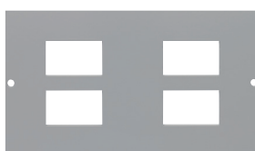
Plate pierced to accept 4 x LJ6C/ RJ45 (Piercings 37.0 x 22.3)
