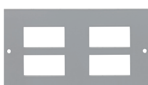
Plate pierced to accept 4 x RW Data/ Alphasnap Units (Piercings 48.0 x 23.5)
