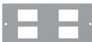
Plate pierced to accept 4 x LJ6C/ RJ45 (Piercings 37.0 x 22.3)
