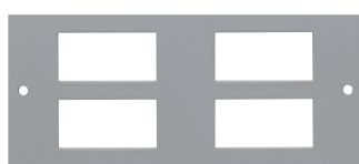
Plate pierced to accept 4 x RW Data/Alphasnap Units (Piercings 48.0 x 23.5)
