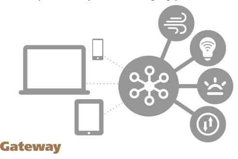
The primary control device; each Gateway coordinates fixtures and sensor components, in the manner that they were grouped together, and provides 24/7 communication with your Audacy Interface. Each Gateway is the "controller" for all of your program inputs.
