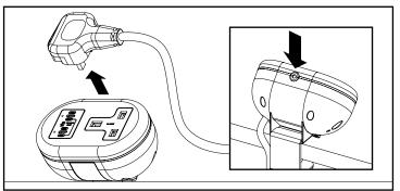
Remove any connected plugs and charging cables. Then press and hold the red circuit breaker with an appropriate tool.
