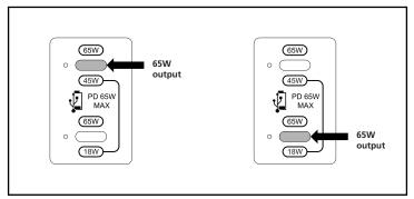
When used in isolation, the top and bottom USB ports deliver a maximum output of 65W.
