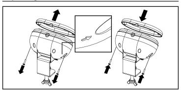
Use a PZ1 screwdriver to remove the 2x fixing screws marked with an arrow on the Caplet body. Remove and replace the fascia. Ensure the fascia is seated correctly on the Caplet. Use the 2x fixing screws to secure the new fascia in place.
