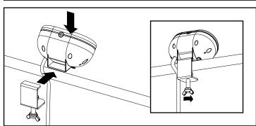
Locate Caplet on the edge of the desk. Offer up the clamp to the rear of Caplet and align to the desk edge. With Caplet held between the clamp and the desk, fully tighten the thumb screw to secure in place.
