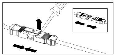
Use an appropriate tool to release the locking mechanism. Carefully pull and separate the male and female connectors.
