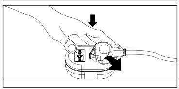
When inserting/removing plugs, take care to support the module where
