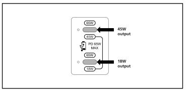
When both ports are used simultaneously, the top USB port has an output of 45W and the bottom port an output of 18W.
