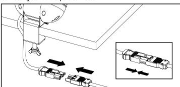
Plug the male 3-pole connector into a female connector. Ensure the attached locking mechanism clicks into place on both connectors.
