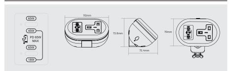
When one USB socket is used, the maximum output is 65W. When both USB sockets are used at the same time, the upper USB socket has a maximum output of 45W and the lower USB socket has a maximum output of 18W. We recommend that higher powered devices, such as laptops, are plugged into the upper socket, for faster charging.
