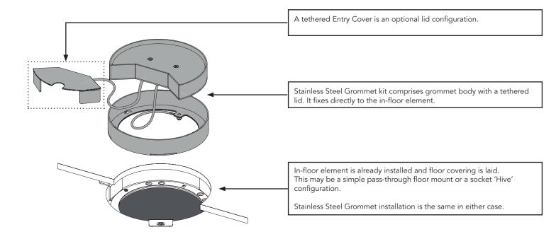
Note that the grommet may be installed prior to the floor covering, so that flooring can be laid accurately up to it.
